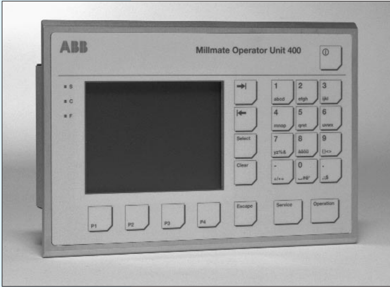
Dimensions (H × W × D) 160 × 235 × 60 mm, IP 65 from the front when mounted on a panel acc. to IEC 529, EN 60-529, IP 20 in all other directions acc. to IEC 529, EN 60-529, weight 1.3 kg
