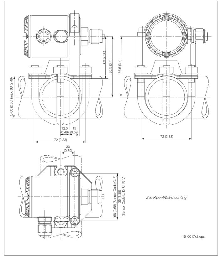
Note: Bracket both for pipe and wall monting provides four holes of 10.5 mm (0.41 in) diameter on square with 72 mm (2.84 in) side
