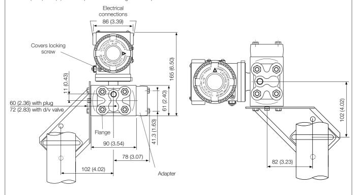
NOTE: Process connection, gasket groove and gaskets are in accordance with DIN 19213. Bolting threads for fixing adapter or other devices (i.e. manifold etc.) on process flange is 7/16in-20 UNF.
