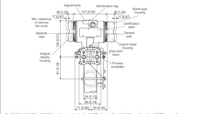
(\*) 51 (2.01), 54 (2.13) or 57 (2.24) mm (in) according to 1/2in 14 NPT adapters fitting 54 (2.13) mm (in) on 1/4in 18 NPT process flange 54 (2.13) mm (in) with low pressure side flange without process connection and drain/vent valve
