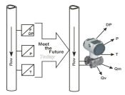
The dynamic mass flow compensation of 267CS is based on AGA 3 and EN ISO 5167:
