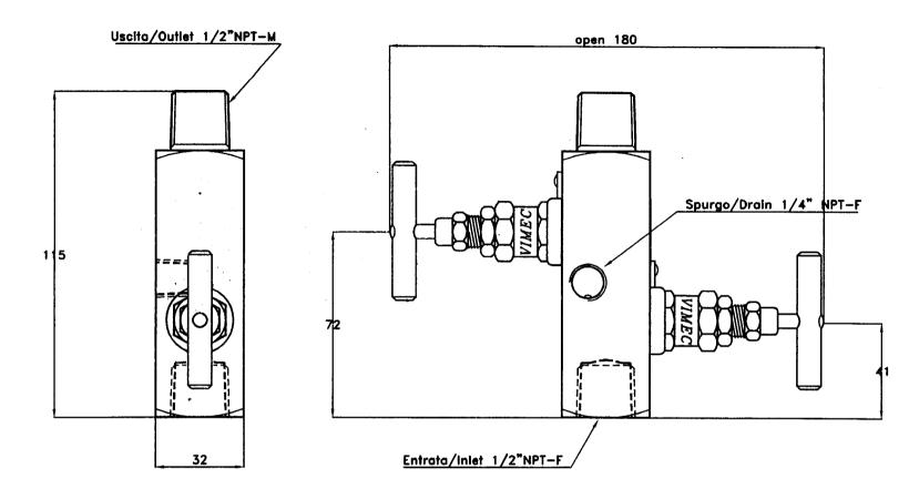
General tollerance on all the drawing  $\pm 0.1$  Millimetrical measuration except different indications
