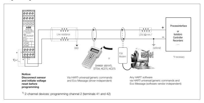
The for all sensor types useable TH01/101 temperature transmitter series is via the new Eco-message-method and the HART-generic/universal driver regarding all transmitter function programmable.
